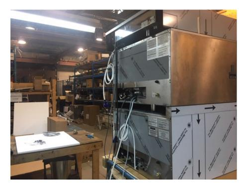
Depending on the model of the top oven, remove the rubber cap from the hood that aligns with the exhaust of the top oven.
