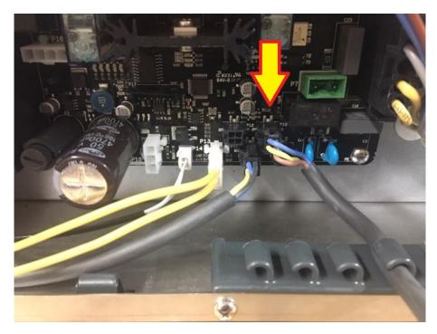
Connect the cable with 2 wires to the unused contacts on the hood contactor. The 2 wires of the same cable must <u>both</u> go into either 'A' or 'B' (**DO NOT CROSS**THEM), the colors are not important.
