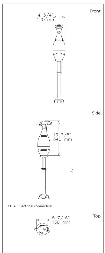
Electric Supply voltage: 602232 (DBP3545U) 110-120 V/1 ph/50/60 Hz **Total Watts:** 0.4 kW Plug type: USA NEMA 5-15P Key Information: External dimensions, 5 7/16" (138 mm) Width: External dimensions, Depth: 4 3/4" (120 mm) External dimensions, Height: 30 1/8" (765 mm) **Shipping width:** 11 7/16" (290 mm) Shipping depth: 27 3/16" (690 mm) **Shipping height:** 7 1/16" (180 mm) **Shipping weight:** 12 lbs (5.29 kg)
