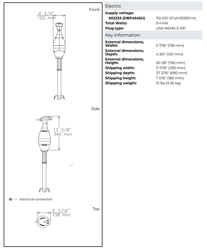
Hand held Mixers Portable mixer+ss tube 453mm/18in, var.speed 450w, nema 5-15p
