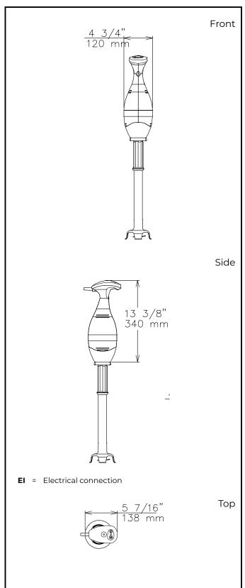
Electric Supply voltage: 602235 (DBP6555U) 110-120 V/1 ph/50/60 Hz **Total Watts:** 0.6 kW Plug type: USA NEMA 5-15P Key Information: External dimensions, Width: 5 7/16" (138 mm) External dimensions, Depth: 4 3/4" (120 mm) External dimensions, Height: 34 1/16" (865 mm) 11 7/16" (290 mm) **Shipping width:** Shipping depth: 27 3/16" (690 mm) **Shipping height:** 7 1/16" (180 mm) **Shipping weight:** 12 lbs (5.42 kg)
