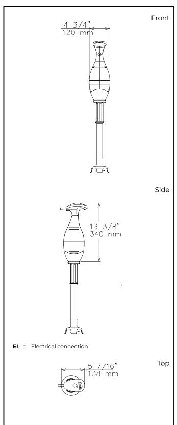
Electric Supply voltage: 602237 (DBP6565U) 110-120 V/1 ph/50/60 Hz **Total Watts:** 0.6 kW Plug type: USA NEMA 5-15P Key Information: External dimensions, Width: 5 7/16" (138 mm) External dimensions, Depth: 4 3/4" (120 mm) External dimensions, Height: 38 " (965 mm) **Shipping width:** 11 7/16" (290 mm) Shipping depth: 27 3/16" (690 mm) **Shipping height:** 7 1/16" (180 mm) **Shipping weight:** 12 lbs (5.61 kg)
