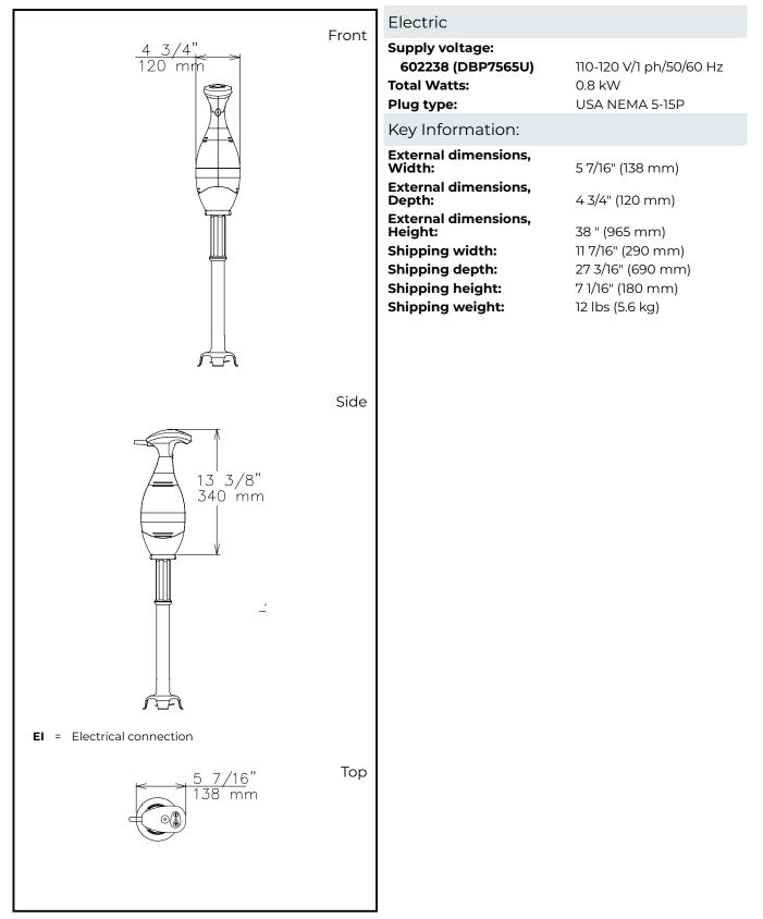
Hand held Mixers Portable mixer+ss tube 653mm/26in, var.speed, 750w, nema 5-15p
