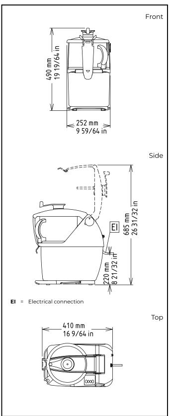
Electric **Supply voltage:** 602242 (DTRK55) 110-120 V/1N ph/60 Hz **Total Watts:** 1.3 kW Plug type: USA NEMA 5-15P Key Information: External dimensions, Width: 9 15/16" (252 mm) External dimensions, Depth: 19 1/16" (485 mm) External dimensions, Height: 19 7/8" (505 mm) Shipping width: 13 " (330 mm) Shipping depth: 32 1/4" (820 mm) **Shipping height:** 23 5/8" (600 mm) **Shipping weight:** 71 lbs (32 kg)
