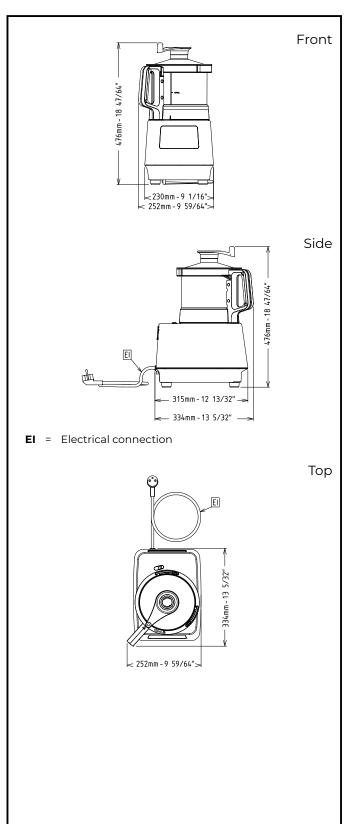
Electric Supply voltage: 602249 (DK36US) 115 V/1N ph/60 Hz **Electrical power, max:** 1 kW **Total Watts:** 1kW Capacity: Performance (up to): Capacity: 3.6 Litre Key Information: External dimensions, Width: 252 mm External dimensions, Depth: 334 mm External dimensions, Height: 476 mm **Shipping weight:** 19.9 kg
