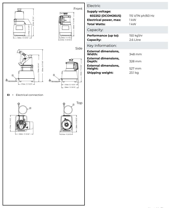
Vegetable Slicer Prep4You Combined Vegetable Slicer/Cutter Mixer 2.6l/2.7qt,1 speed, 2discs incl.,1000w, nema 5-15p The company reserves the right to make modifications to the products without prior notice. All information correct at time of printing.
