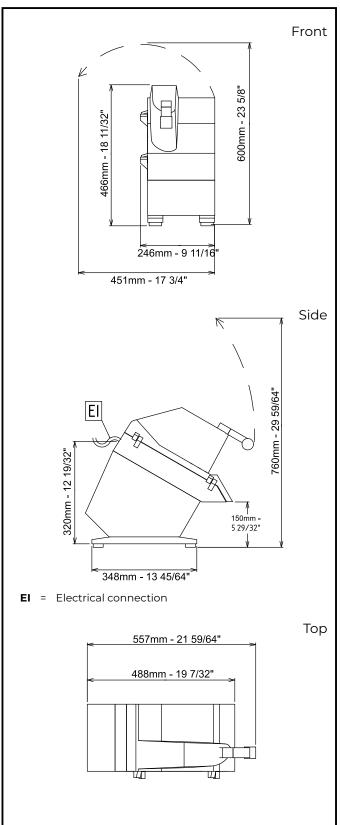
Electric Supply voltage: 602256 (DTR24SNU) 115 V/1N ph/60 Hz **Electrical power, max:** 0.6 kW **Total Watts:** 0.6 kW Capacity: Performance (up to): 450 kg\hr Key Information: External dimensions, Width: 246 mm External dimensions, Depth: 557 mm External dimensions, Height: 466 mm
